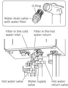
2. With a bucket ready, remove the water drain valves.
